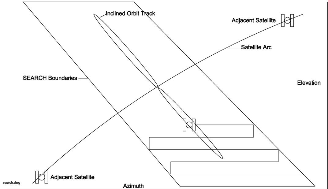
The automatic search may be disabled via the Search Enable CONFIG mode item. If the automatic search is disabled, the user is prompted to manually position the antenna on the satellite.
