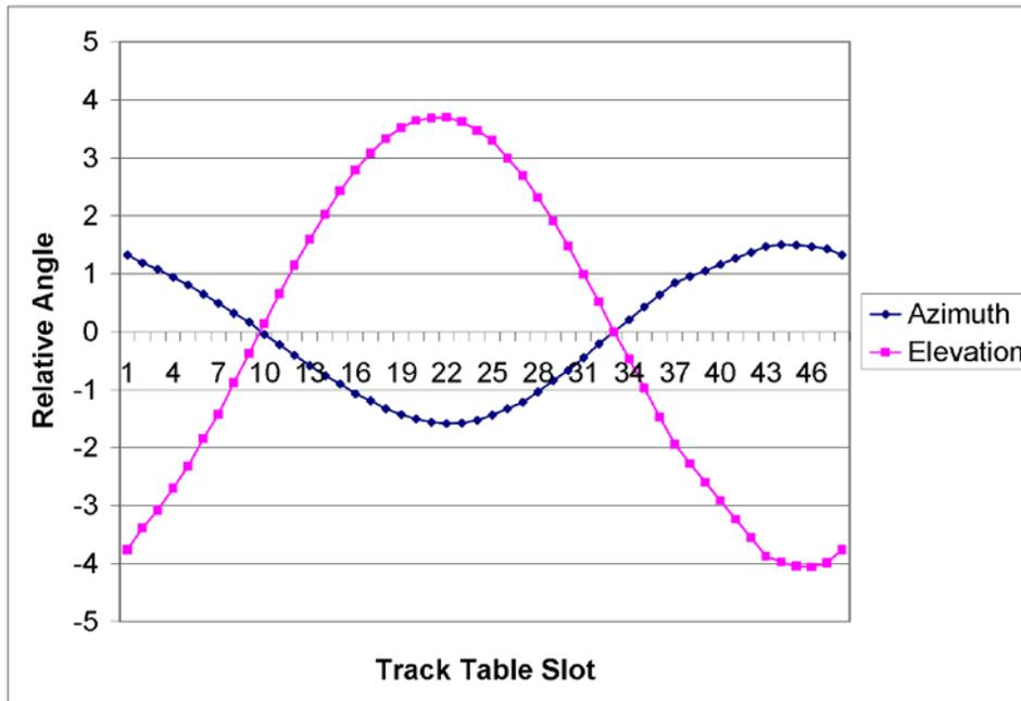
During a `step_track` operation, the controller peaks the antenna by monitoring the received signal strength. Signal strength information is available to the controller via the signal strength input. The signal strength input accepts a DC signal generated by the AGC circuits of a satellite receiver, or by a beacon receiver. The signal strength setup and configuration procedure is described in section 4.1.11 of the baseline manual.
