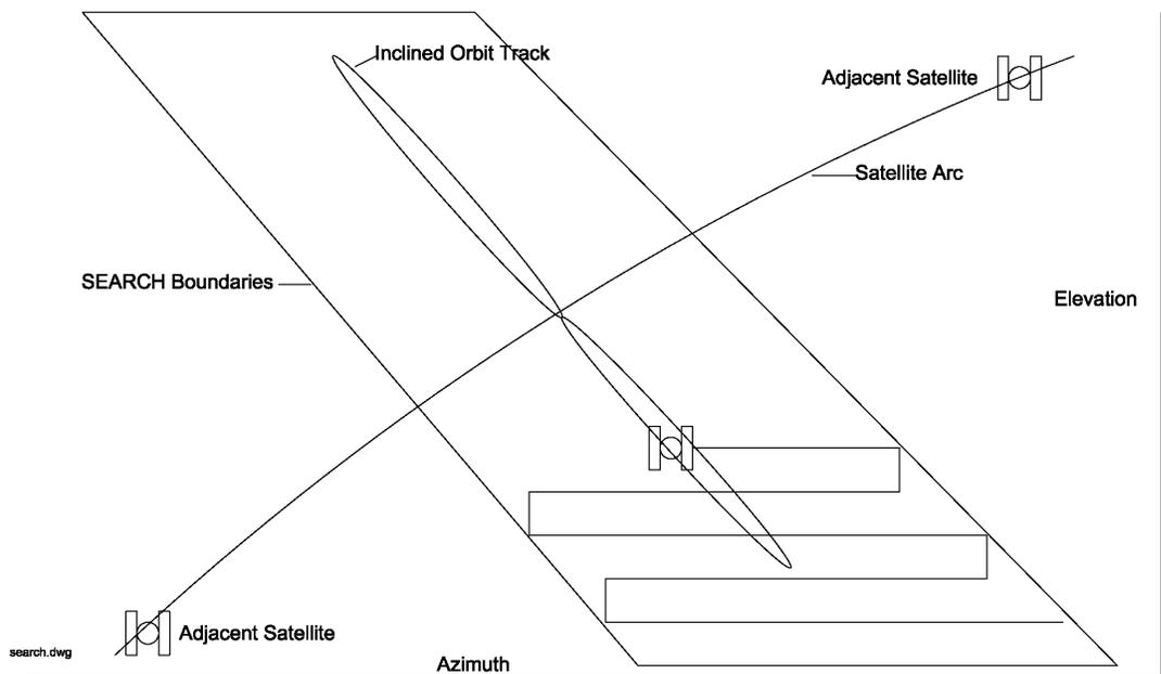
is calculated based on the satellite inclination angle specified by the user when the track is initiated from SETUP mode. The width (or short dimension) of the parallelogram is specified by the *Search Width* parameter entered via CONFIG mode. The *Search Width* has a range of values of 1 to 10, with 1 specifying the narrowest search window and 10 specifying the widest window. The default value of 3 is adequate for most situations.
