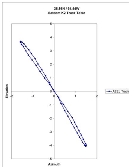
The exact shape of the pattern varies with the longitudinal position of the satellite and the place on the earth from which the satellite motion is viewed. To estimate the height and width of an inclined orbit satellite's motion as viewed from the surface of the earth, a good approximation is to multiply the results of the equations above by 1.2.
