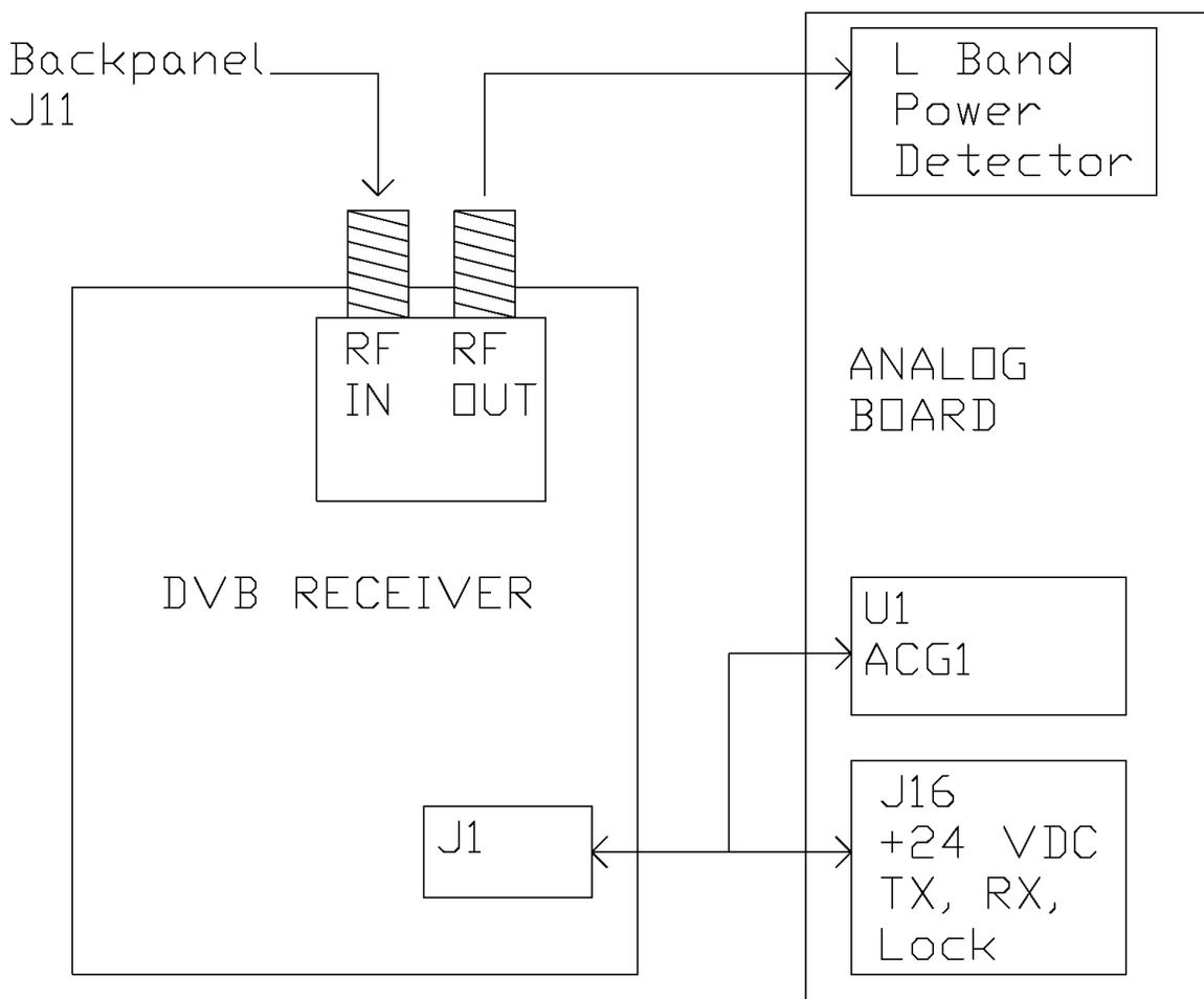
Power and serial communications will be mechanized via a cable between the DVB's J? connector and the J16 connector on the analog board.
