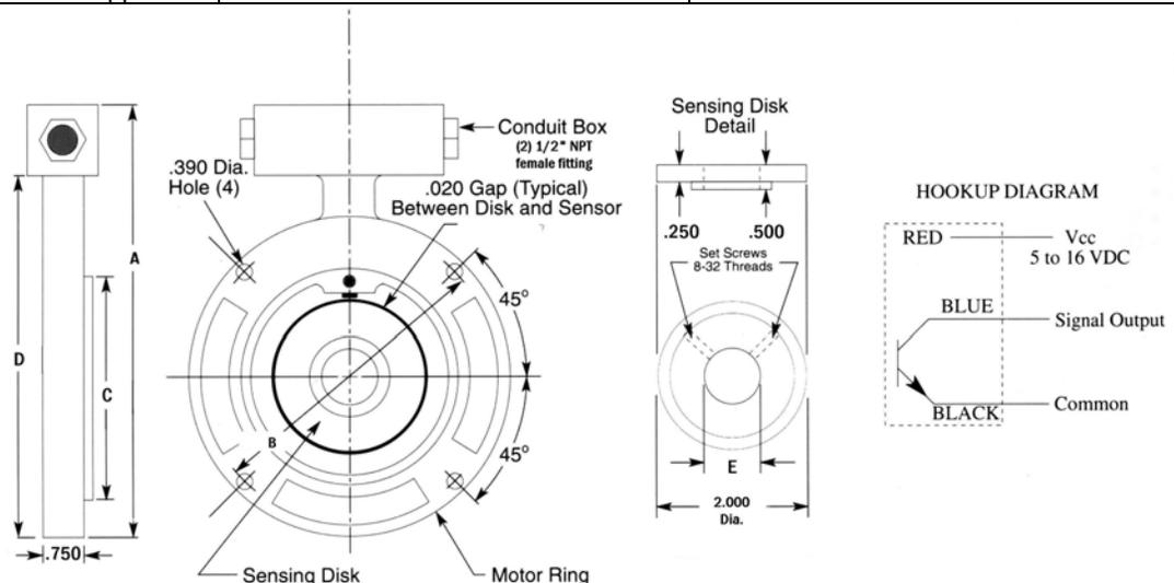
NOTE: To interface sensor to controller, use a shielded triple (18-22 AWG) with bare drain wire, such as Belden 8772.
