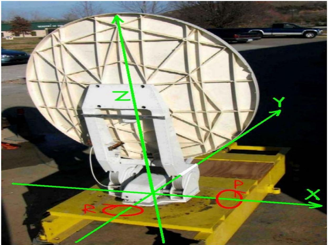
To correctly estimate antenna heading and to properly sense platform tilt, the TAC must be placed orthogonal to the antenna platform and must be calibrated while the platform is level.
