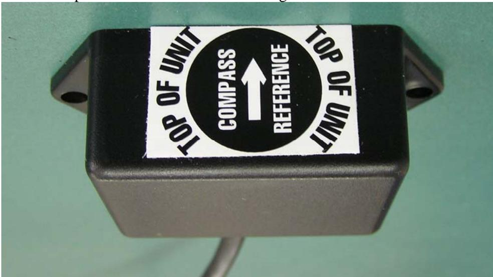
The user should choose horizontal or vertical mounting orientation according to where it is most convenient to mount the box while satisfying the requirement that the top of the box must be able to be maintained level by moving the elevation axis as the mount is rotated in azimuth. This requirement will typically mean purchasing a horizontal mount box when the unit will be attached to a structure that will be horizontal when the antenna is in the DEPLOY position.
