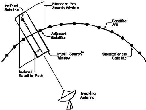
Note that the inclination of the satellite increases with time. The maximum rate of increase is approximately 0.9 degrees per year. As the inclination increases, the width of the figure 8 pattern will also increase. This has two implications for system performance. One, the maximum signal loss due to antenna misalignment will increase with time, and two, the antenna must have range of motion sufficient to accommodate the greatest satellite inclination that will be encountered.
