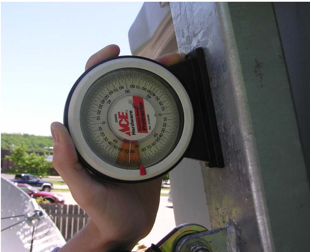
Figure 20 – Inclinometer Placement to Set Down Limit
