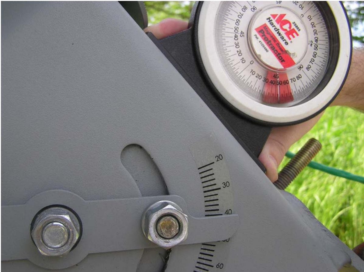
Figure 18 – Placement of Inclinometer for Adjustment of Latitude Angle
